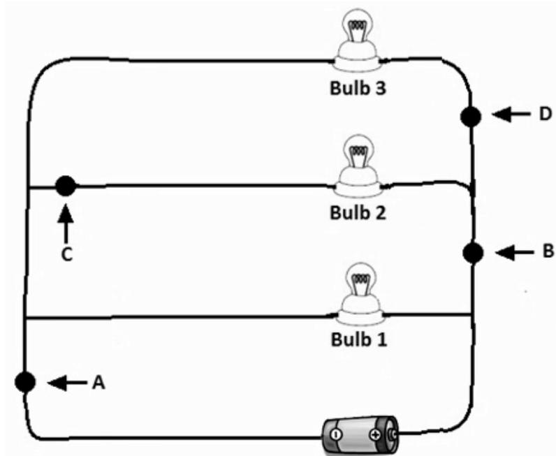
9. Where should you put a switch so that bulb 2 and bulb 3 can be switched on and off, but bulb 1 will stay on all the time?
